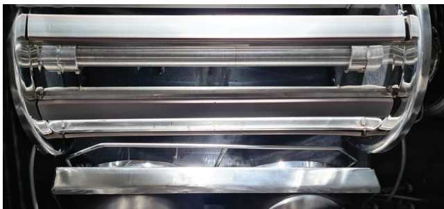
lifting reel of the long tube dyeing machine
