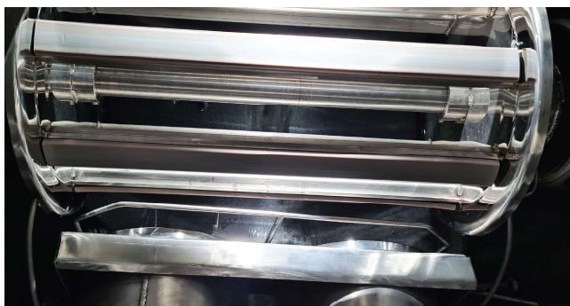
lifting reel of the long tube dyeing machine
