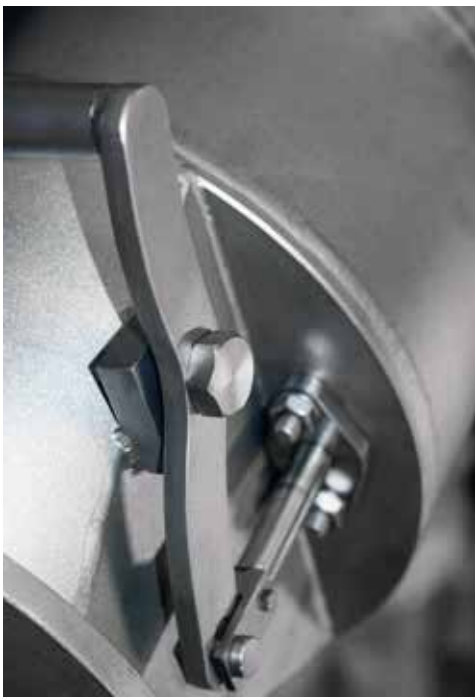
mechanic for adjustment of the nozzle gaps
