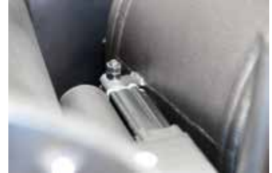
pneumatic for adjustment of the nozzle gaps
