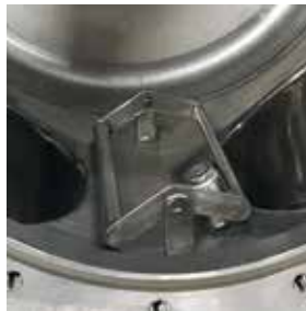
magnetic device to prevent the fabric from getting stuck
