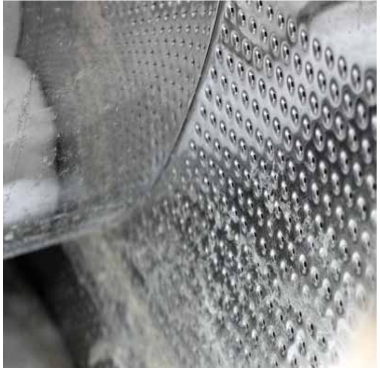
perforated side wall in the treatment chamber
