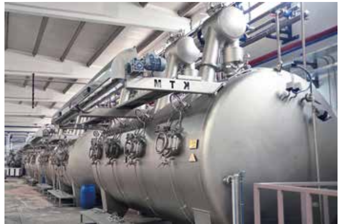
RAPIDDYE® machines in a dye house
