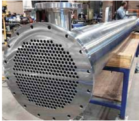
inside view of the main heat exchanger
