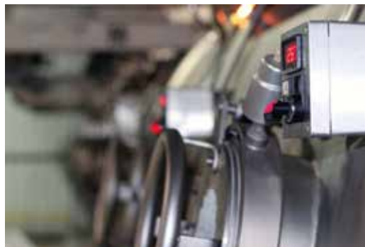
pneumatic piston for security lock
