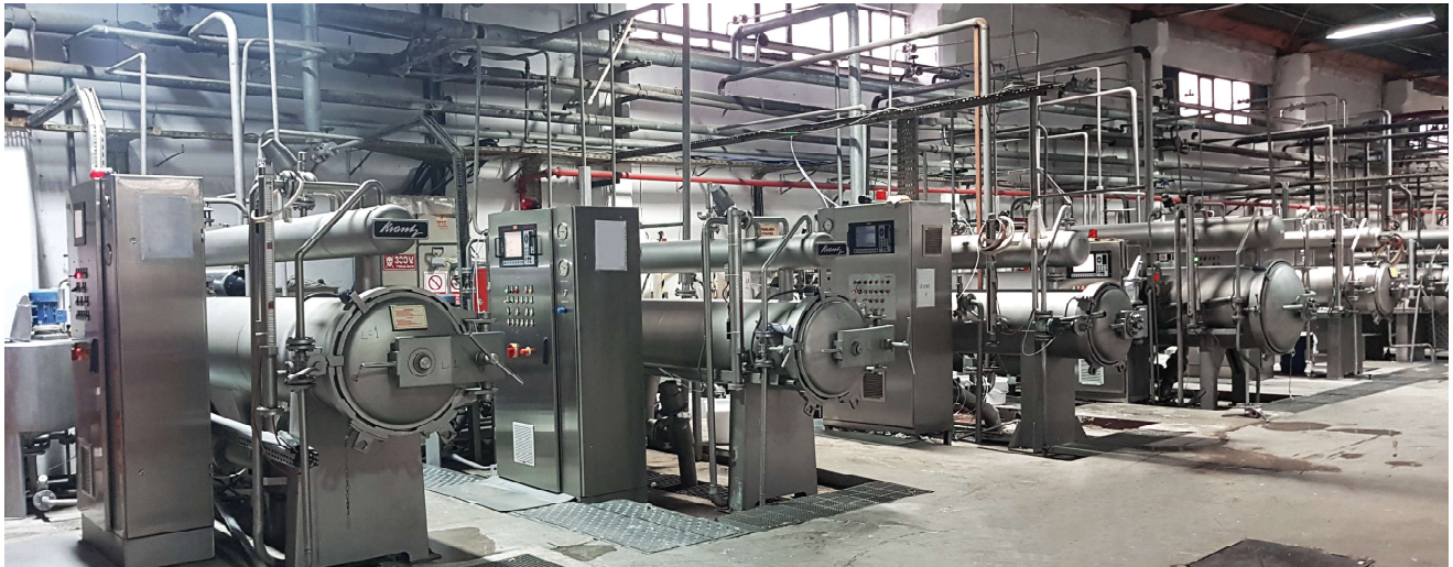
Kranz BEAMDYE-B-HT ® technical side & top view
